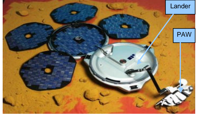
▲ Beagle 2 lander with instruments on its robotic arm
