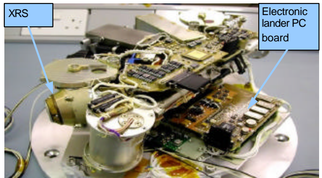
▲ Top view of PAW (position adjustable workbench)
